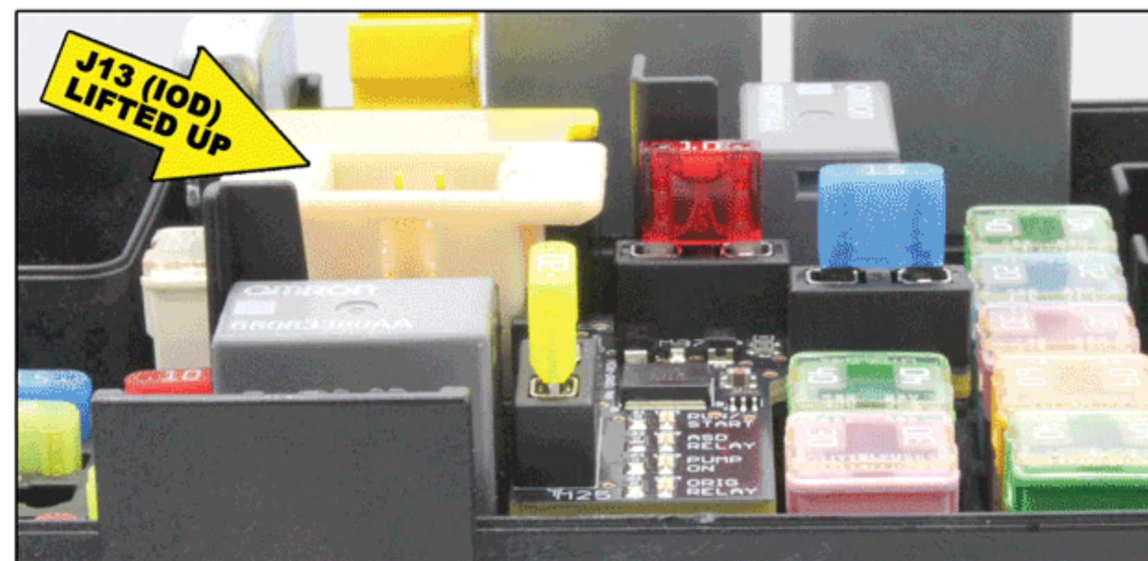
Figure 4 - Fully main seated circuit board
