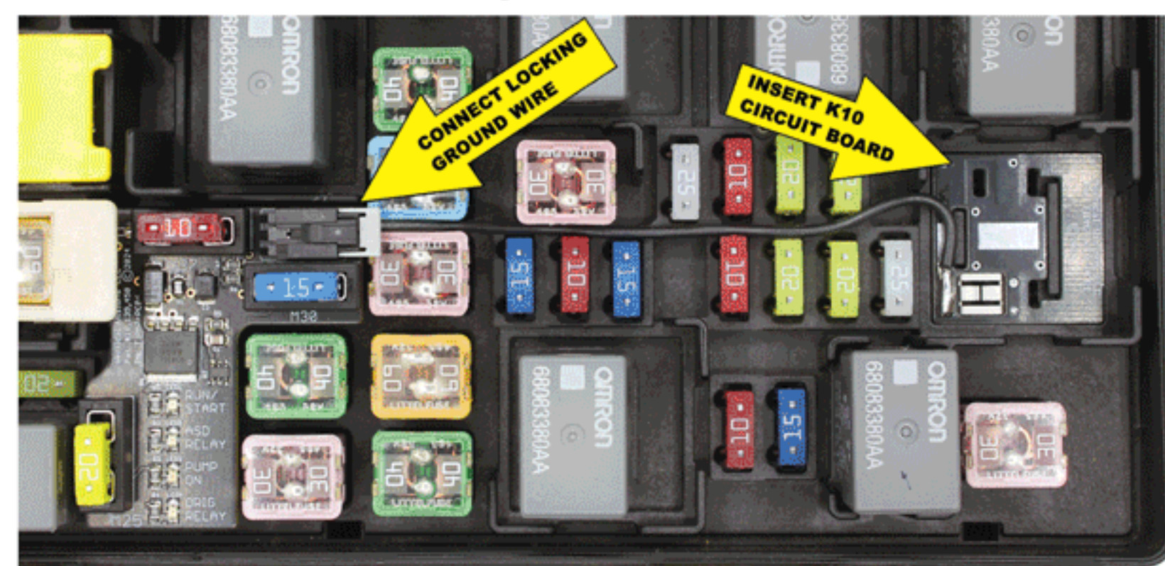
Figure 5 - Insert small K10 circuit board into the TIPM
